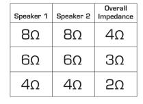
Warning: The  $3\Omega$  (ohms) and  $2\Omega$ (ohms) settings can damage the Casaman.
