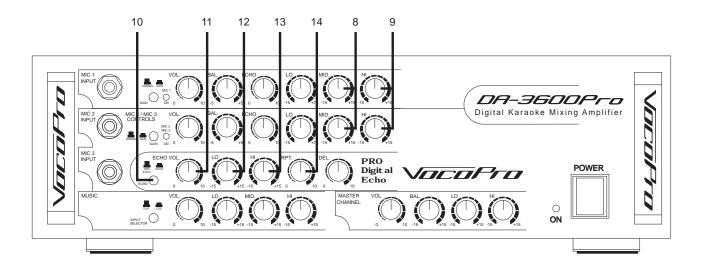
8. MID. control – This control increases/decreases the amount of MID-RANGE frequency response applied to the MIC channels. Turn clockwise to increase the MID-RANGE frequency response and counter-clockwise to decrease the MID-RANGE frequency response.
