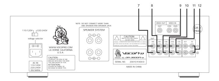
7. MIC OUTPUT jacks – These jacks export MIC 1, 2 and 3 OUTPUT only, bypassing the source audio signal in order to provide connection to vocal effects units. Connect a paired RCA-ended patch cable from these jacks to appropriate INPUT jacks on the vocal effects unit.
