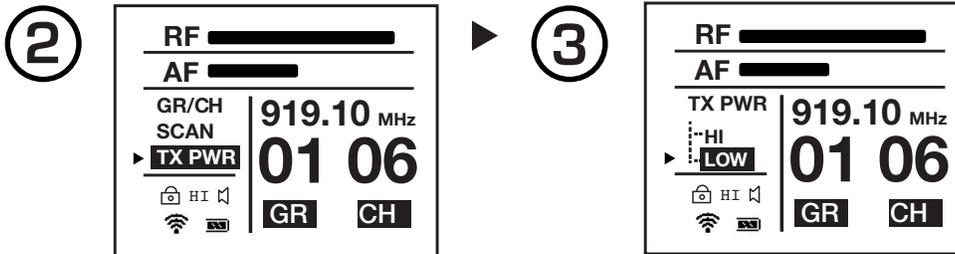
4. Once output power has been modified, hold the microphone IR sensor in line and within 4 inches of the IR sensor located near the display.
