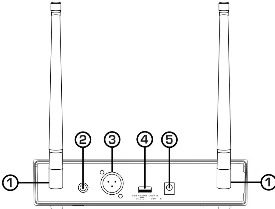
1. Antenna – These receive the RF/AF transmission from the microphone.
