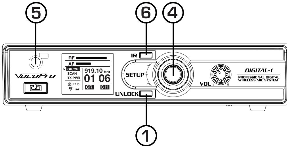
1. Press and hold the unlock button the access the Menu.
