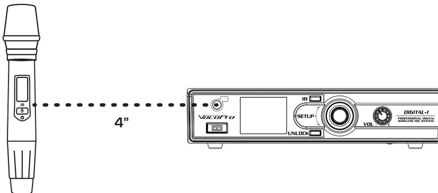
5. Press the IR button to communicate the new power level to the microphone.
