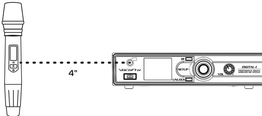
6. Press the IR button to communicate the new frequency to the microphone.
