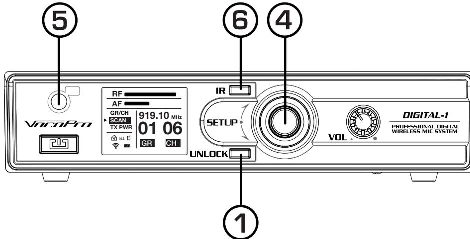
1. Press and hold unlock button to access the Menu.
