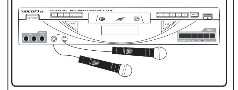
Connect up to two microphones to the DVX-880 PRO, by connecting a 1/4" cable to the MIC 1 and 2 inputs on the DVX-880 PRO.
