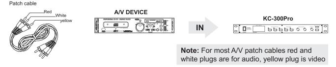
**(b)** To connect an AUXILIARY device, you will need either a line-level patch cable (red and white RCA plugs), or XLR cables. Plug one pair of RCA/XLR plugs to the appropriate AUDIO OUT jacks on your auxiliary device. Plug the other pair of RCA/XLR plugs to the AUX IN jacks on the KC-300Pro.
