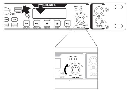
5. Once Mic and Music are balanced, reduce the Record Level knob until the REC LEDs are constantly green. This indicates optimal recording level has been achieved.
