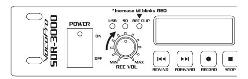
3. Slightly reduce the record level until the REC CLIP LED is a constant green (no RED). You now have an optimal recording level.
