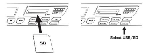
4. Remove an SD card by pushing the card forward until it clicks and pushes out. NOTE: The SDR-3000 cannot accept cards larger than 4GB or SDHC cards.
