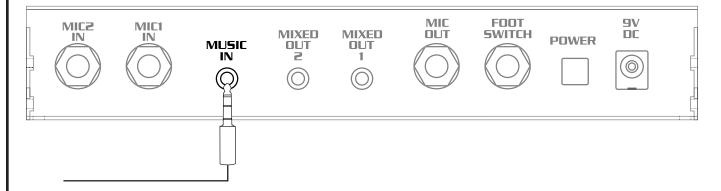
2. Connect a microphone to Mic 1 or 2 In using a 1/4" cable
